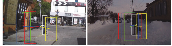
Figure 7: Failure cases. The failure forecasts are often caused by randomness of 2D trajectory mutations during prediction period. The same color coding (see Fig. 4) is used.
